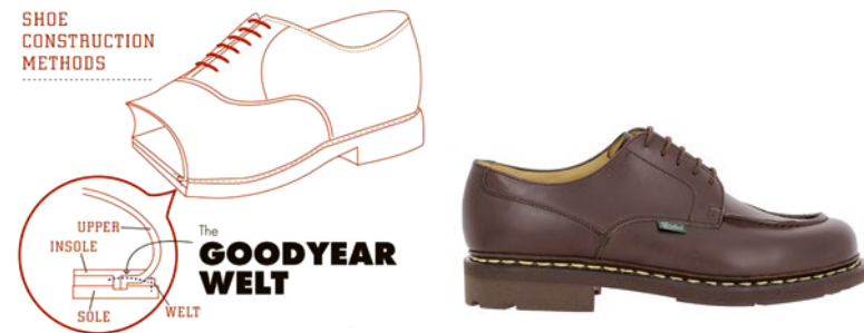
Example of Goodyear welted shoes: ©Paraboot
