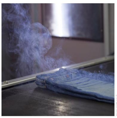
Levi Strauss & Co has invested in improving the environmental impact of garment manufacturing. A collaboration with Project F.L.X. (future-led execution) will change the finishing process of denim from hand detailing to automated laser in order to reduce chemical use.
