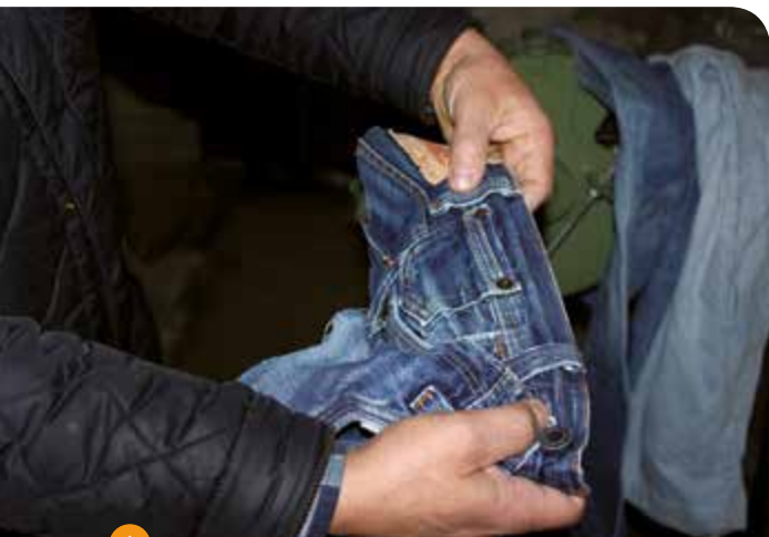
Cutting of jeans, removal of hard items to prepare the fraying of material.
