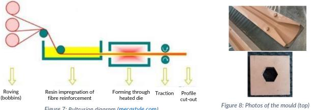
Figure 7: Pultrusion diagram (mecastyle.com)
