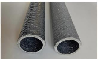
Figure 6: Tubes with a shiny finish (left) and a rough finish (right)
