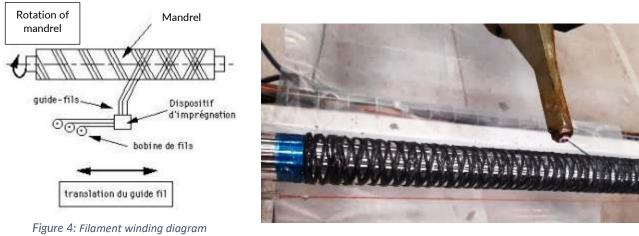
Figure 5: Filament winding with the recycled yarn
