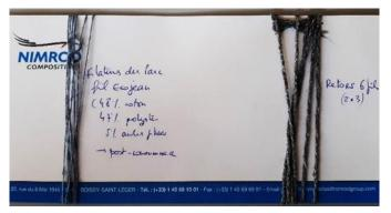
Figure 2: Standard ECOJEAN yarn (left) and retwisted ECOJEAN yarn (right)
