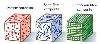
Figure 1: Diagram showing composite types (Boufaida, 2015)
