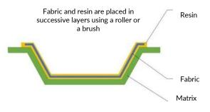
Figure 10: Composite manufacturing by impregnation (ouest-composites.com)
