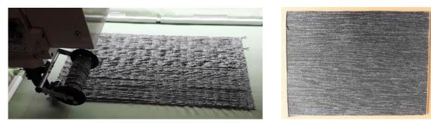
Figure 3: Manufacturing of the yarn/epoxy composite plate for mechanical characterisation
